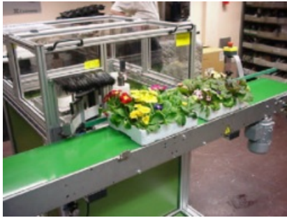
Codeway Green Machine printing and applying labels to plant trays
